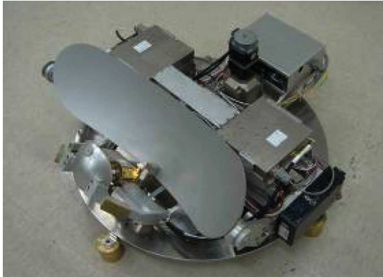
Fig. 12. Photo of the entire assembled mobile antenna system.
