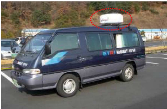
Fig. 16. Antenna system installed on the test van.
